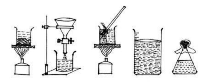
Boiling potato slices Filtering through cheese cloth Boiling Potato extract + Dextrose+ Agar
